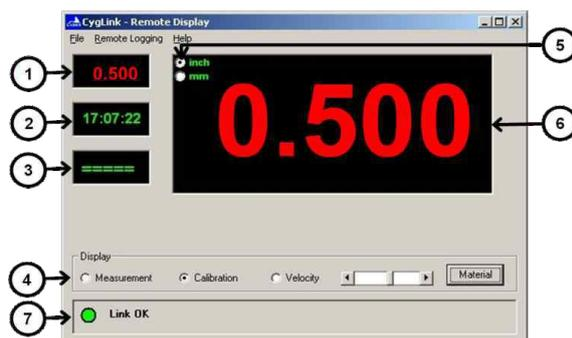
1. Displays the last thickness measurement value
